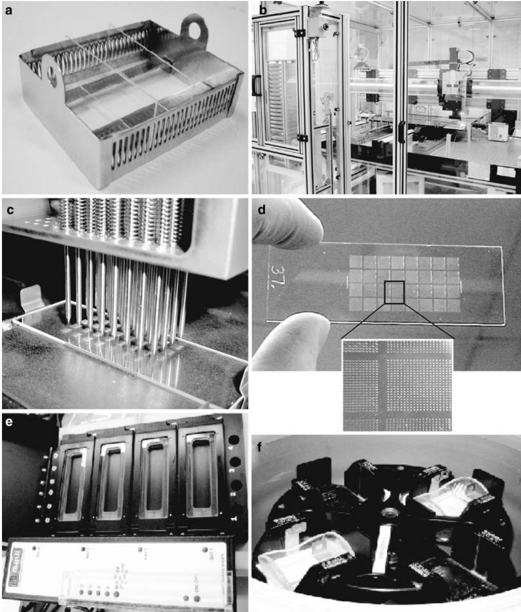
Fig. 2. Selected instruments and materials used in microarray wet-lab. (a) Stainless steel slide rack used during cleaning and poly-L-lysine coating of glass slides. (b) A robotic spotter or arrayer placed in a printing chamber to provide a dust-free environment. (c) Solid steel printing pins spotting probes on a glass slide. (d) A microarray slide with visible printed spots, as a result of the dried salt deposition on the glass surface, prior to post-processing. The probes are spotted orderly in grids with high precision and density (Inset). (e) The MAUI™ hybridization system, which allows four slides to be hybridized simultaneously in a controlled environment. (f) A centrifuge with a swing-out rotor and microtiter plate holders that can accommodate staining rack is required for rapid drying of microarray slides.
